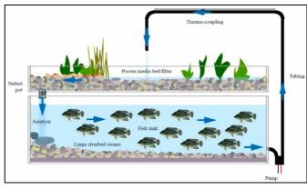
**Fig. 3:** A model of aquaponics (Adapted from:https://images.app.goo.gl/Ty5KbD1KnzfdzDnm6)
