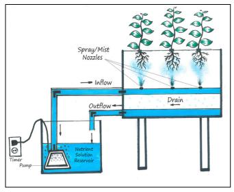
**Fig. 4:** A model of <u>aeroponics</u> (Adapted from:https://images.app.goo.gl/b6PwS2zWwCta7qHv7)
